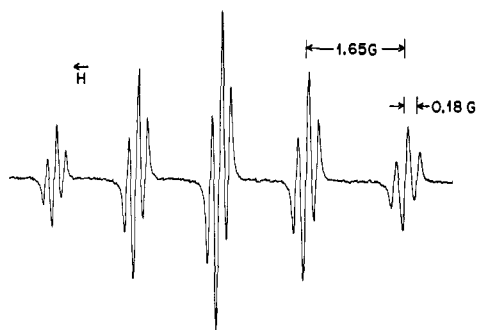
Figure 8. Spectrum during photolysis at 32.5° of aqueous 8.77 mM parabanic acid containing 5% isopropyl alcohol. The pH was 3.90. This is designated spectrum III in the text.
